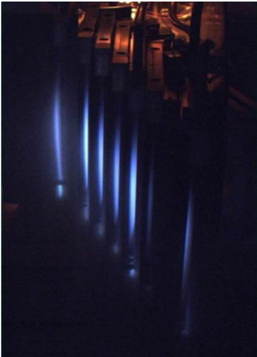
Figure 2: Electromagnetic separation of ^{96}\text{Ru} at ESIPP. Image courtesy of ORNL.
