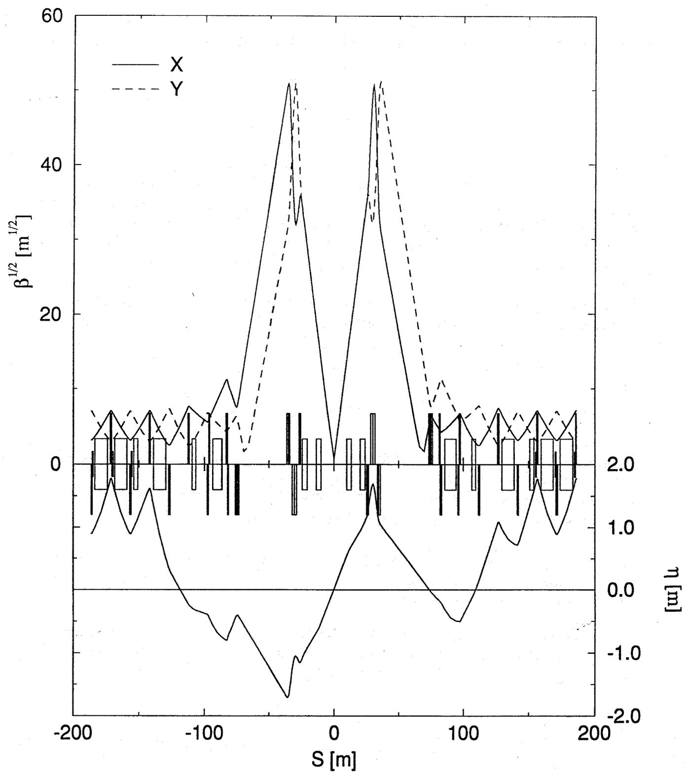
Figure 1. The beta and dispersion functions of a RHIC insertion at  $\beta^*=0.5\text{m}$ .
