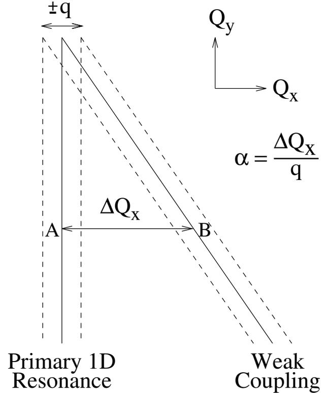
Figure 3: Modulational diffusion resonance structure. The resonance separation is parameterized by  $\alpha$ , which is the horizontal tune distance  $\Delta Q_x$  scaled by the primary resonance half width – the tune modulation depth  $q$ .
