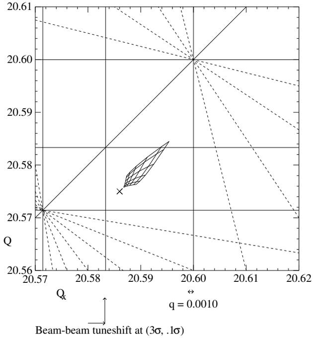
Figure 4: The tune plane for 1992 Tevatron parameters, showing the 5th, 7th, and 12th order resonances. The nominal working point is indicated by a cross, and the beam-beam footprint for  $\xi = 0.005$  at two collisions is shown. Footprint contours of constant amplitude range from  $0.1\sigma$  to  $5.1\sigma$  in  $1\sigma$  increments.
