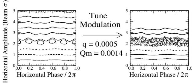
Figure 2: The transition to “thick layer” chaos in horizontal phase space when tune modulation is turned on in the presence of a  $Q_x = 3/5$  resonance. These results come from a simulation of the Tevatron with two beam-beam collisions of strength  $\xi = 0.0005$ , offset by  $\Delta x = 0.1\sigma$ .
