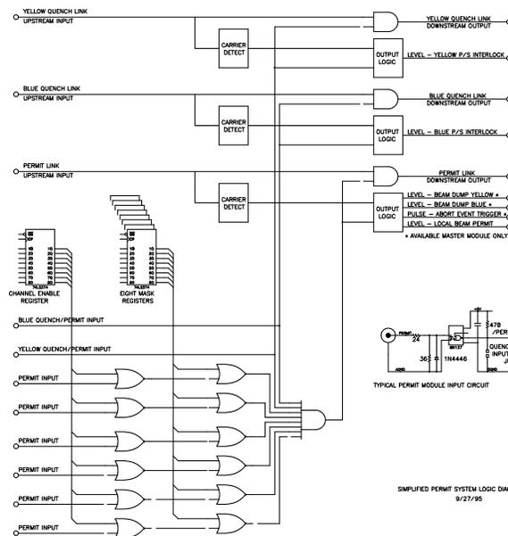
Figure 2: Beam and quench protection permit links logic diagram.
