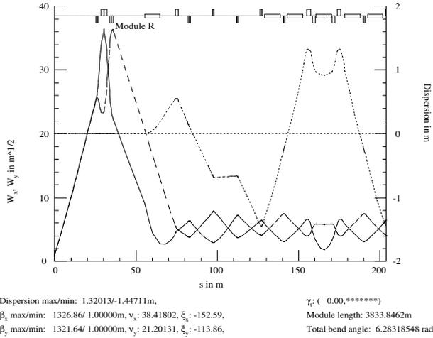
Figure 1: Isochronous RHIC lattice-IR with one FMC module.
